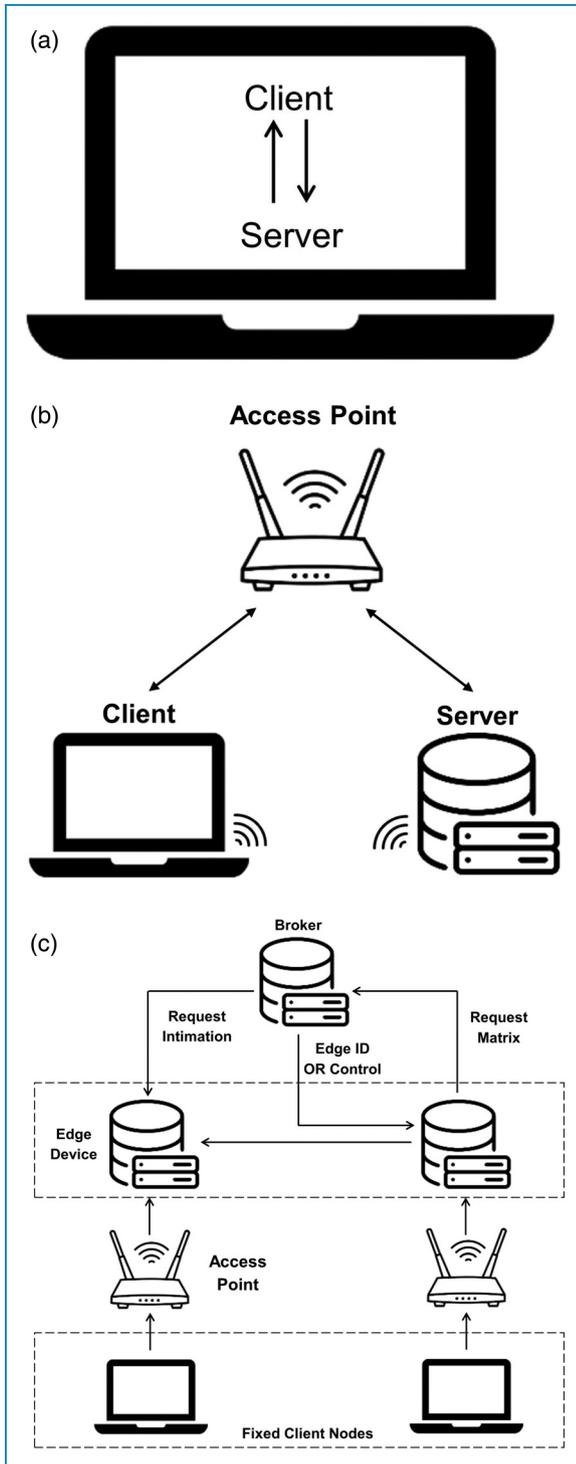
**Figure 3.** Use cases for the experimental setup. (a) First use case: Client and server are both executed on the same machine; (b) Second use case: Client and server are executed on two separate machines; (c) Third use case: Edge federation comprising two fixed client nodes, two edge devices, and a broker.
