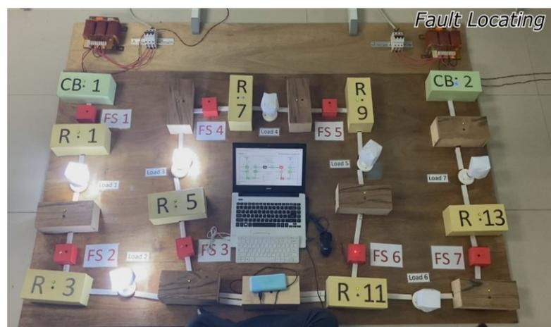
**Figure 13.** Hardware situation when the fault on Line 11 (FS6) is triggered.
